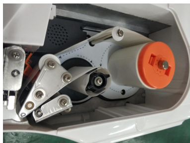
e. Wind the paper on the paper winding shaft for fastening and fasten the print head.
