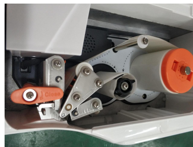
f. Press [FEED] button to roll paper.
