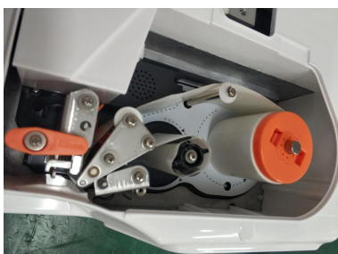
g. Restore the paper stop block and close the dust cover.
